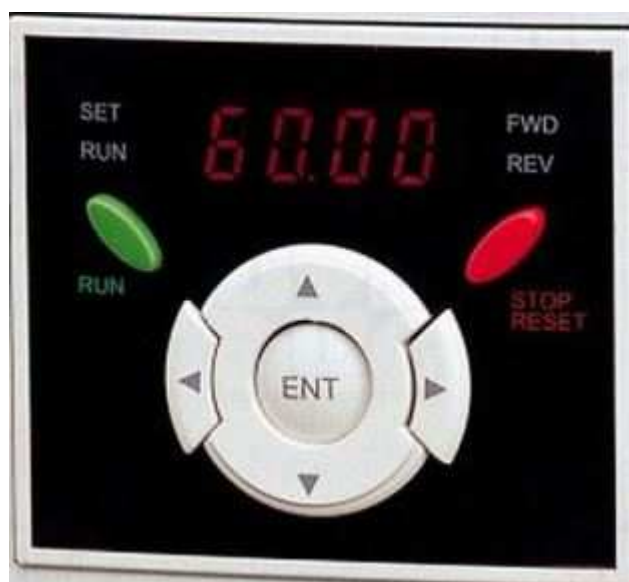
[Rys. 1] Inverter Panel
